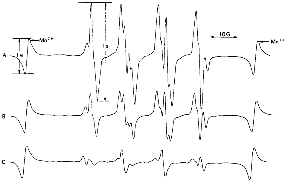
FIGURE 2 ESR spectra of DMPO-OOH spin adducts. DMPO spin adducts shows the superoxide anion ( O_2^- ) generated by the reaction of Hypoxanthine (HX) and Xanthine oxidase (XOD). A standard reaction mixture contained 0.5 mM HX, 0.96 mM DETAPAC, 7.5 mM DMPO, 0.1 U/ml XOD and various concentrations of standard SOD or sample (50 \mu l) in phosphate buffer (pH 7.8). Spectrum A is without SOD. B is 6.25 units/ml of SOD. C is 50 units/ml of SOD.
